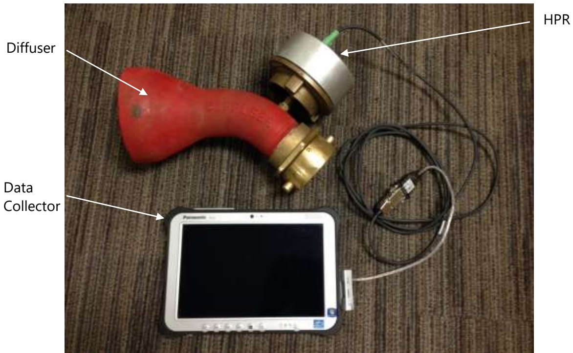
Figure 5-4 – Diffuser, HPR, and Data Collector
